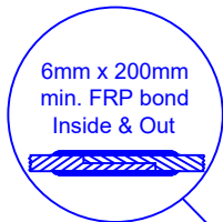
SECTION-JOINT DETAIL
