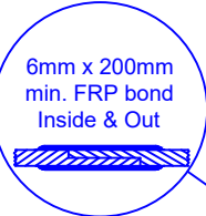
SECTION-JOINT DETAIL
